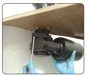
4. Tighten the two screws ( Nm/ 71in-lb). Be sure to align the flange.
