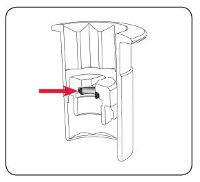
Before screw the central screw, check the correct position of the o-ring in the assy socket and apply Harken® grease.
