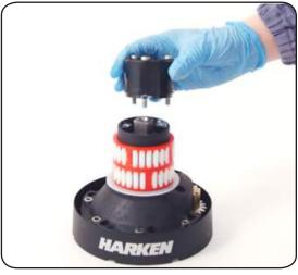
6. Completely unscrew the three screws  $n^{\circ}$  29 and remove the stripper arm support  $n^{\circ}$ 23
