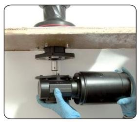
3. Position the reduction gear and motor
