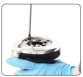
4. Unscrew the three screws n°29 (~4Nm/35 in-lb)
