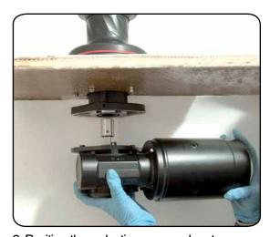
3. Position the reduction gear and motor
