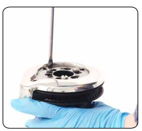
4. Unscrew the three screws n°27 (~4Nm/35 in-lb)
