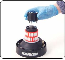
6. Completely unscrew the three screws  $n^{\circ}$  27 and remove the stripper arm support  $n^{\circ}$ 21
