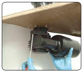
4. Tighten the two screws ( $^{\sim}$ 8 Nm/ 70in-lb). Be sure to align the flange.
