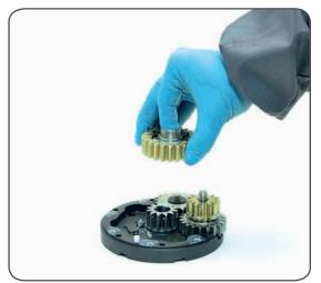
12. Remove gear n°6 and remove the pawls n°4. To facilitate the operation press the spring against the pawl with a blade.
