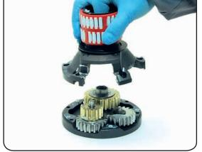
10. Remove the drum housing n°14 Important: washer n°11 may remain inside the drum support!
