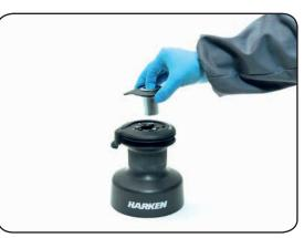
2. Slide off the socket  $n^\circ 25$  and the cover  $n^\circ 26$
