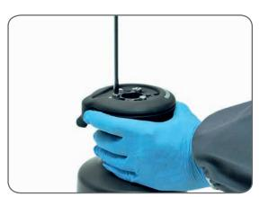
3. Unscrew the three screws n°24 (∛4Nm/35 in-lb)
